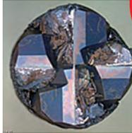
Welding occurred during the second stage of machining (machining stopped).
