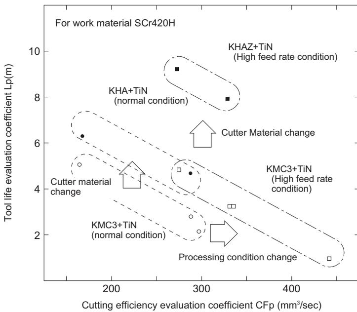
Fig.12 Tool life and machining efficiency
