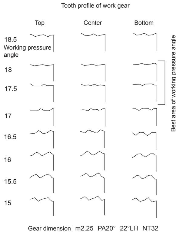
Fig. 12: Tooth shape simulation results
