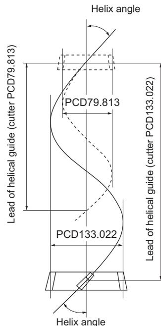
Fig.8 Number of cutter teeth and lead of helical guide
