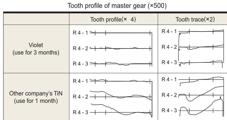
Master gear : Number of teeth 45 Tooth width 19mm Powder metallurgy Hss
