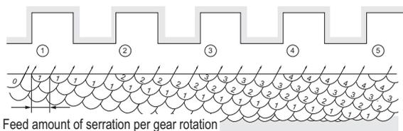
Each serration cutting edge uniformly effects on tooth flank, and cutting amount is uniform
