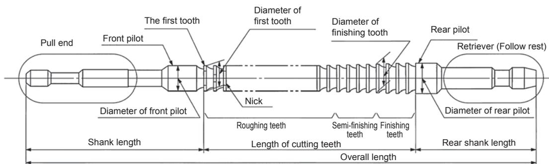
Fig.1 Parts names of pulling broach
