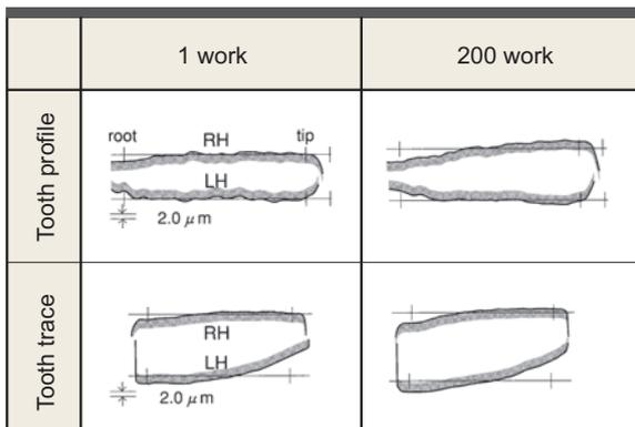
Fig.7 Profile and lead error
