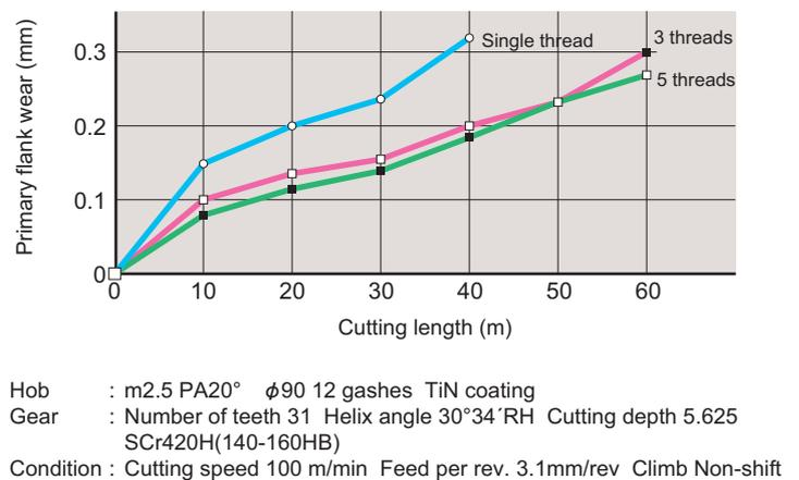
Fig.7 Number of threads and primary flank wear
