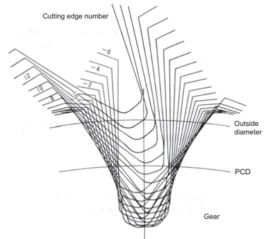
Fig.2 Gear generation line chart
