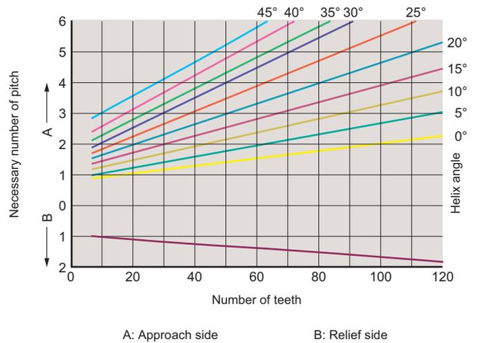
Fig.10 Necessary length of hob for both sides from center line of hobbing machine
