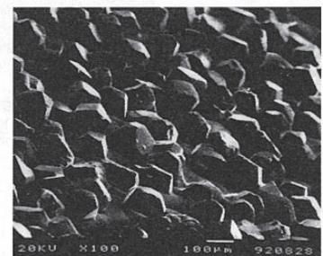
Photo. 1 SEM photograph of tooth surface of dressing gear
