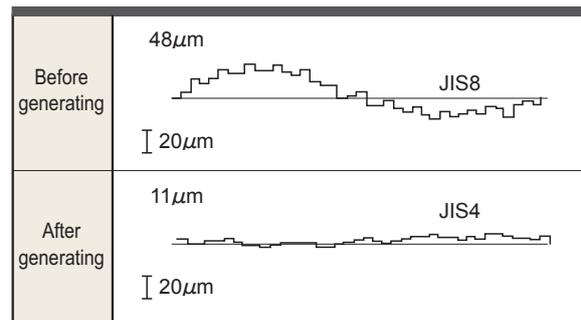
Fig.8 Accumulative pitch error
