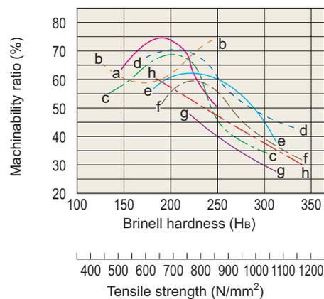
a is the structural steel of 0.3%C or below, cold deformed and drawn.
