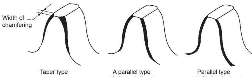
Fig.3 The chamfering shape
