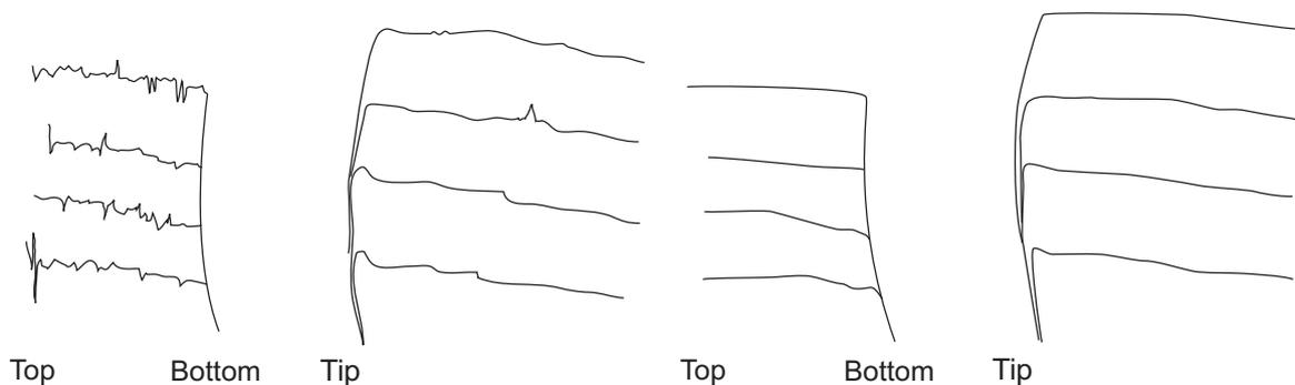
Tooth trace of work gear (x 500.2); tooth profile of work gear (x 500.4); tooth space runout of shaving cutter is 75 μm
