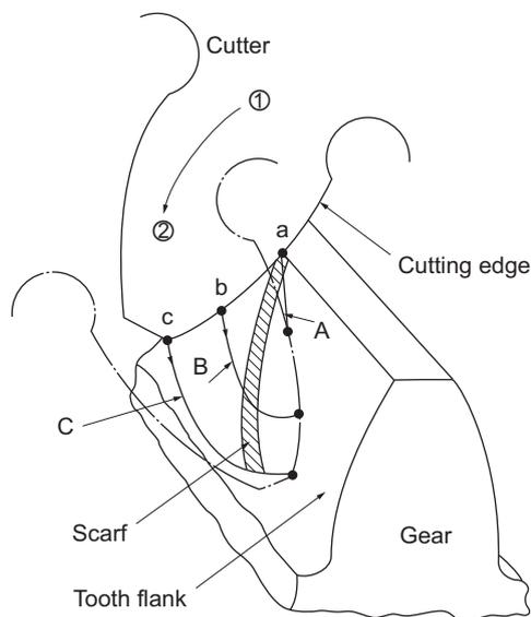
Fig.2 Movement of cutting edge on gear tooth flank
