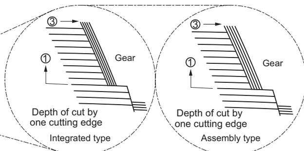
Fig.8-2 Comparison of machining allowance between integrated and assembly types (Enlargement of part A in Fig.8-1)
