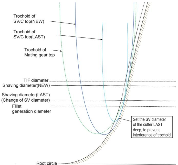
Fig.14 Trochoid chart (without interference of cutter LAST)
