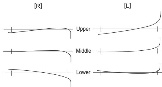
Fig.5 Tooth profile of gear after honing
