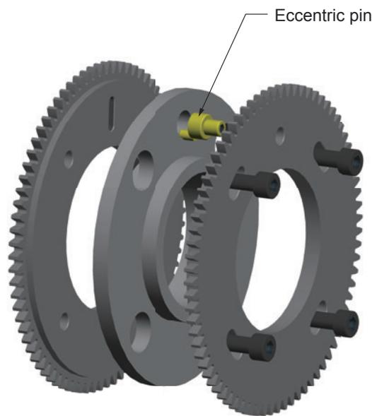
Fig. 5 Phrasing cutter with eccentric pin
