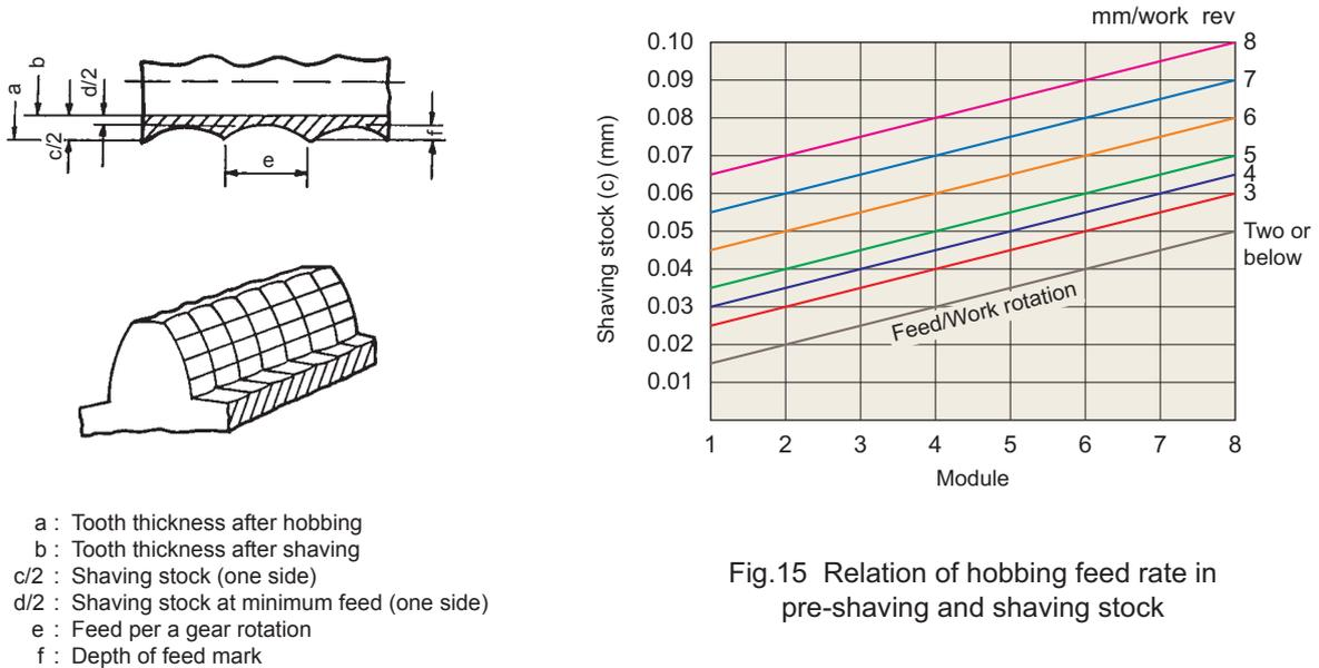
Fig.15 Relation of hobbing feed rate in pre-shaving and shaving stock
