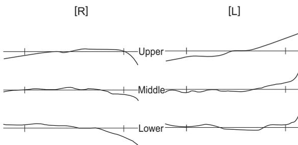
Fig.4 Tooth profile of dressing gear ground
