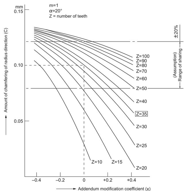
Fig.5 Relation of number of teeth, addendum modification coefficient and amount of chamfering
