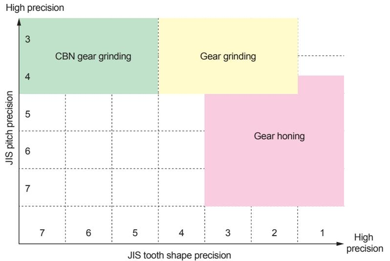
Cutting method for various gears and target
