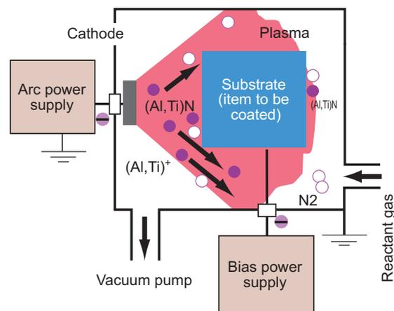
Concept chart of arc-ion plating device
