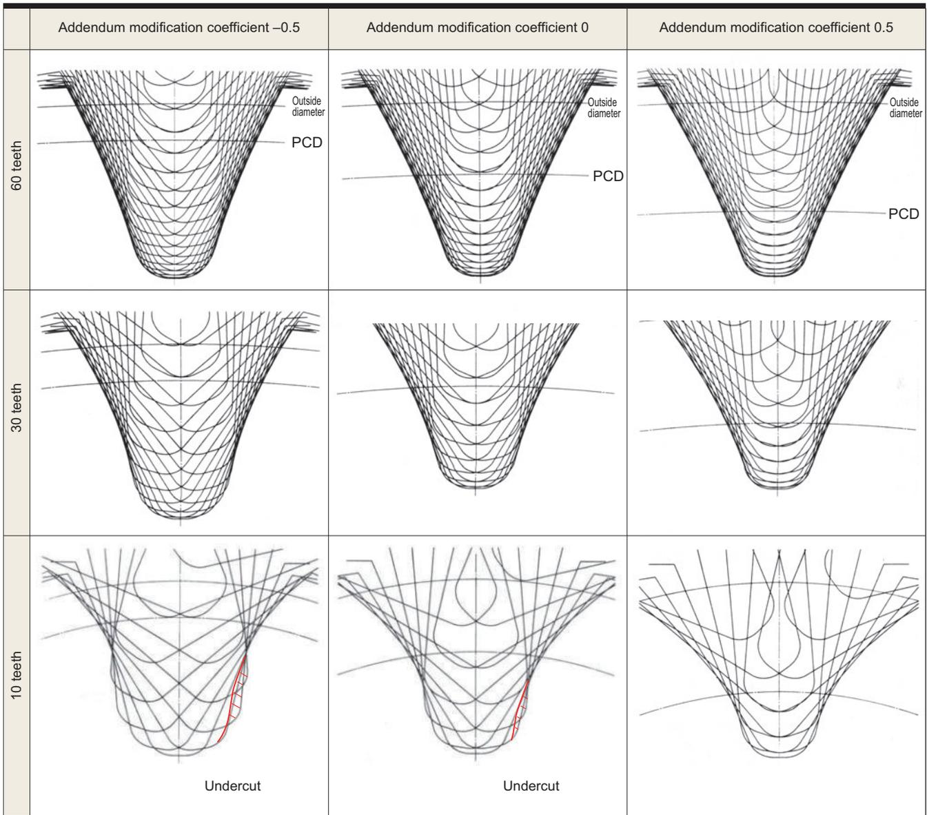
Gear ···  $m=1$ ,  $\alpha=20^\circ$ ,  $\beta=30^\circ$ , Cutting depth 2.4
