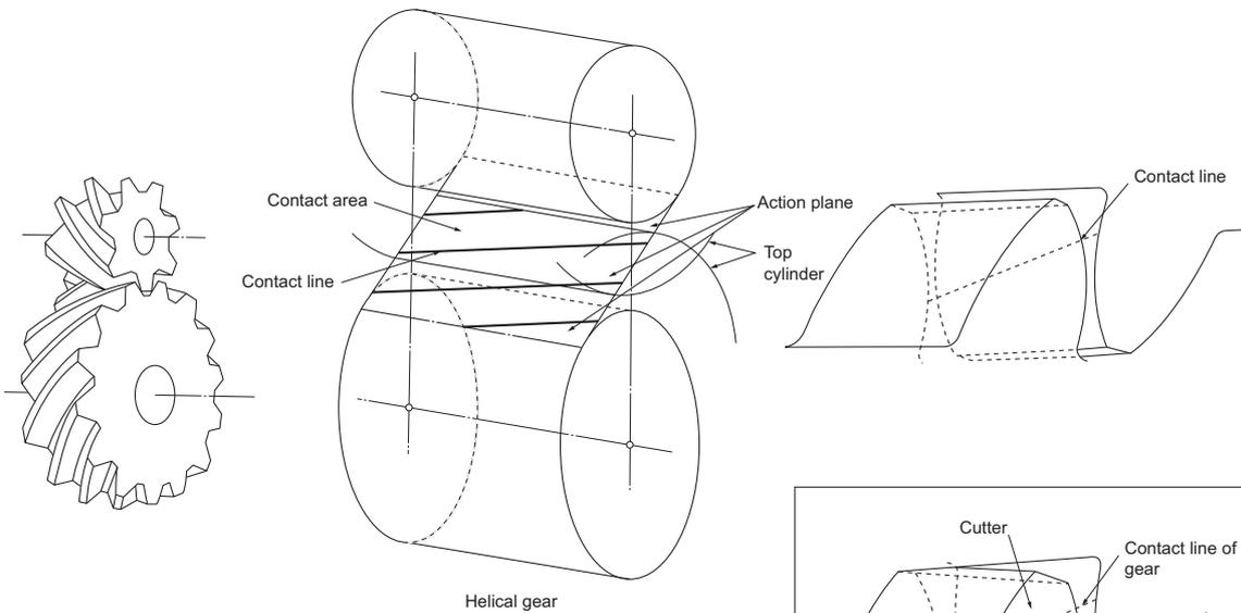
Contact of spur gears and helical gears
