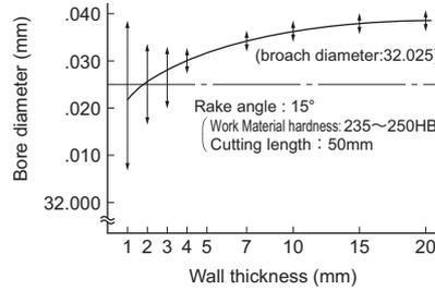
Fig.21-1 Relation between hole diameter and wall thickness
