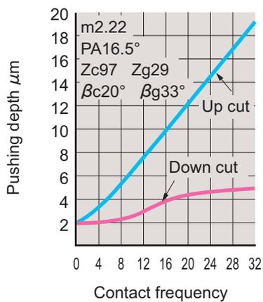
Shows press-in depth for pressing with same force as given in Fig. 17
