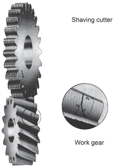
Fig.1-1 State of mating of shaving cutter and work gear
