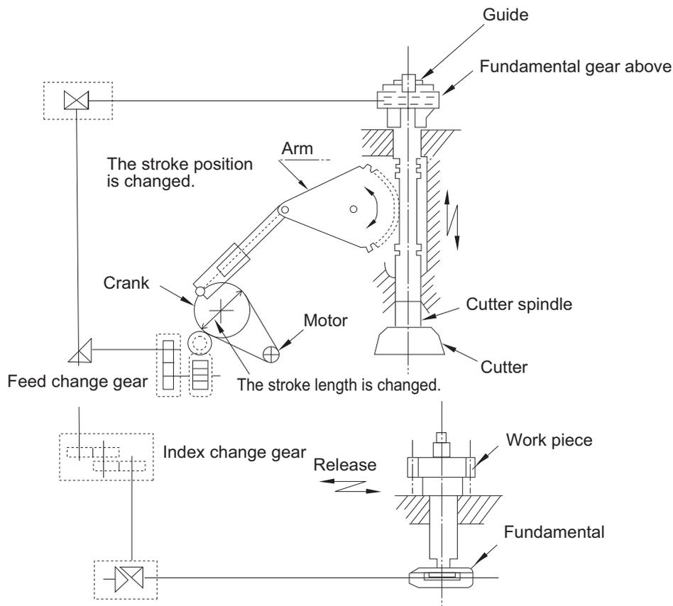
Fig.5 Mechanism chart of gear shaper
