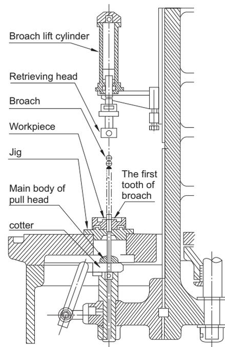
Fig.12 State of broach pulled out
