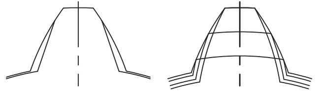
Fig 16-1 Land leaving method      Fig 16-2 Back taper method
