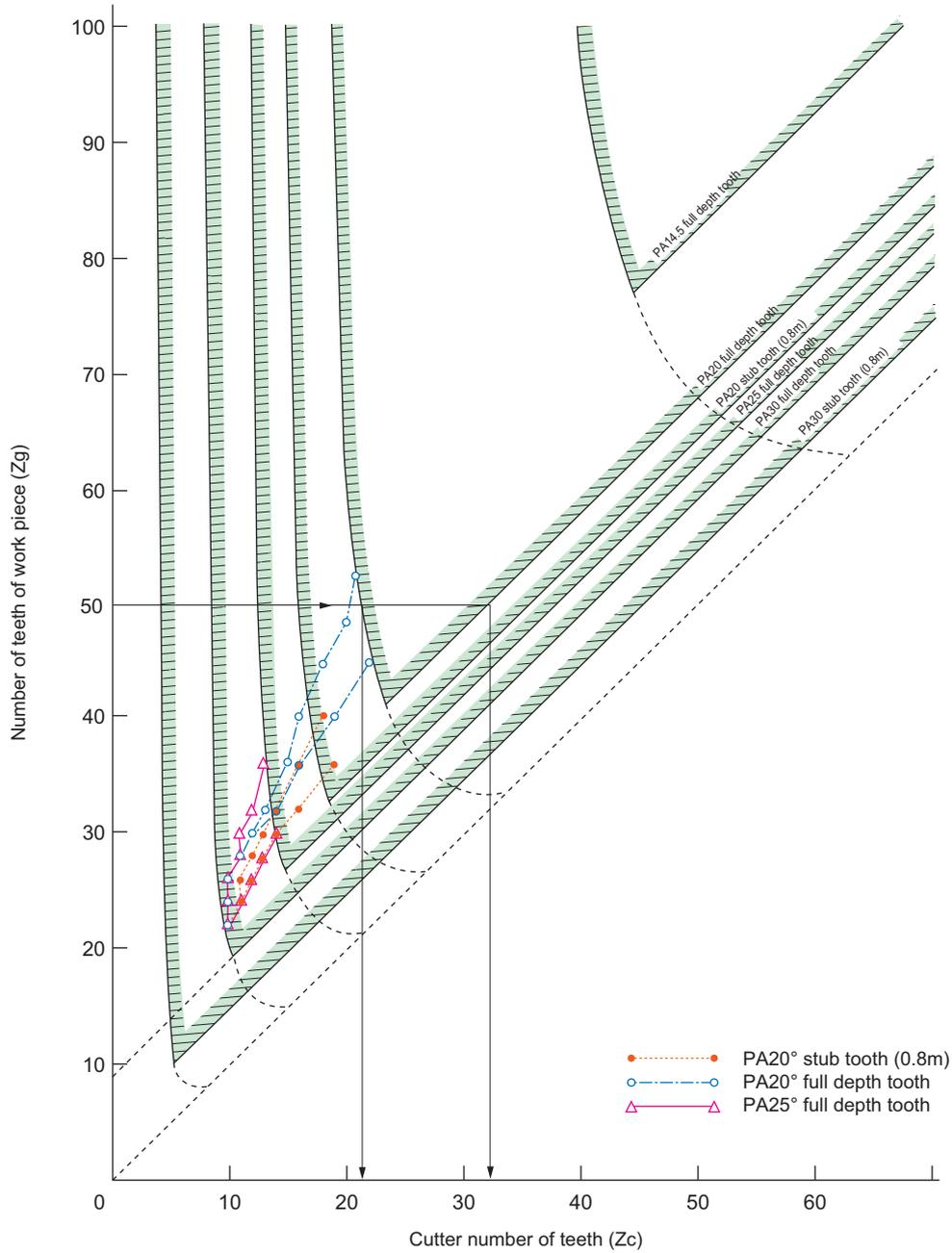
Fig.9 Standard number of teeth selection with shaper cutter for internal gear
