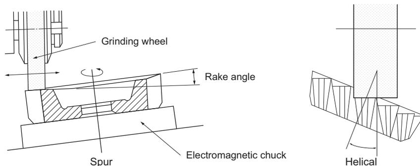
Fig. 11 Shaper cutter regrinding method
