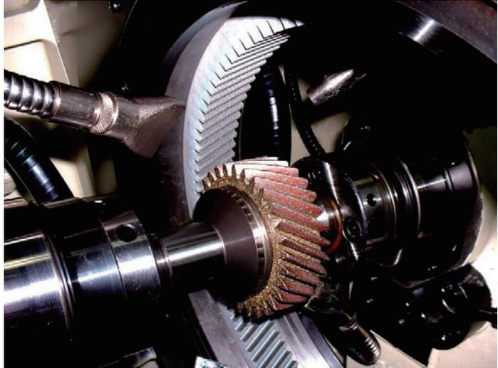
Diamond dressing gears have the same shapes as work piece gears as shown in Fig.1.
