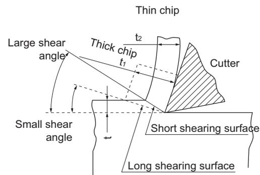
Fig.19 Shear angle and chip thickness
