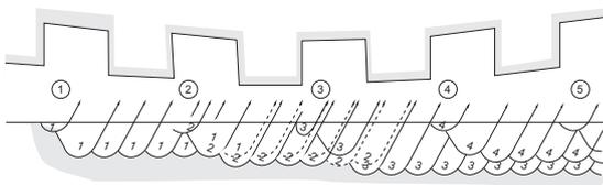
Nonuniform amount of cutting for each serration cutting blade
