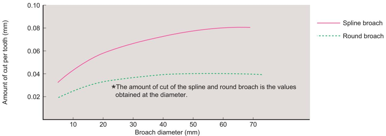
Fig.14 Standard amount of cut per tooth in machining of steel
