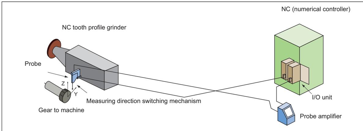
Fig.11 Sketch drawing of gear tester
