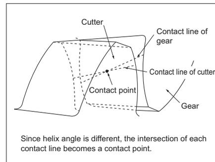
Since helix angle is different, the intersection of each contact line becomes a contact point.
