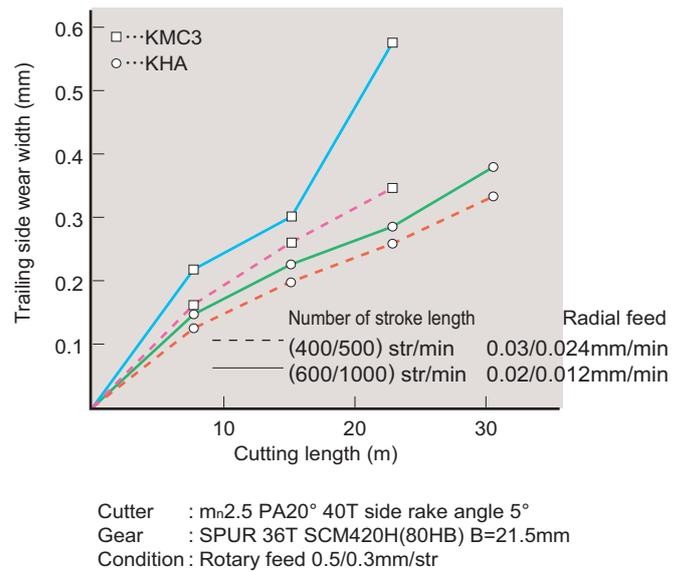
Fig.13 Effect of powder metallurgy HSS
