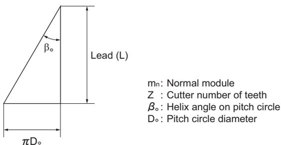
Fig.7 Lead of helical guide
