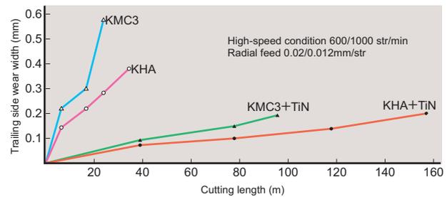
Cutter : m<sub>n</sub>2.5 PA20° 40T side rake angle 5°
