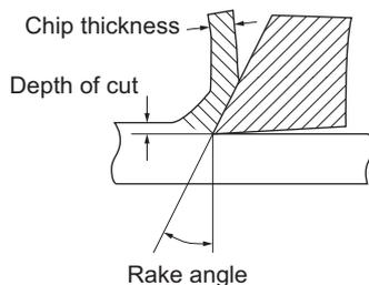
Fig.18 State of chip generation
