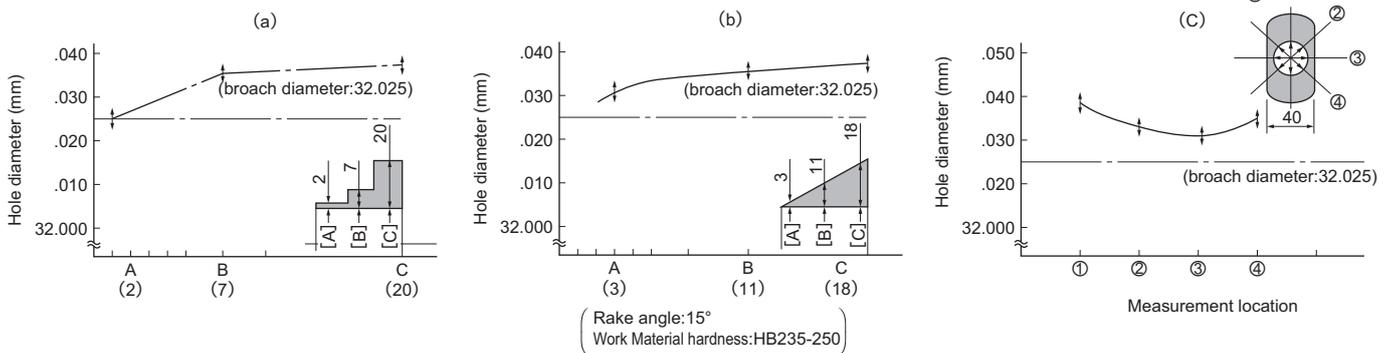
Fig.22 Bore diameter and the special shape wall thickness (Each point in the graph is an average value of five works)
