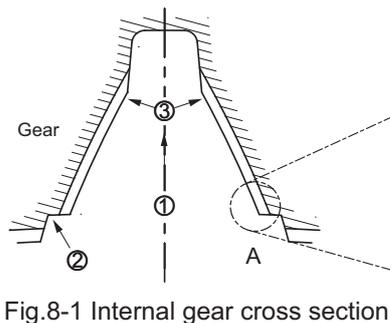
Fig.8-1 Internal gear cross section
