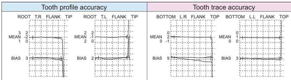
Fig.9 Tooth profile accuracy of machined gear
