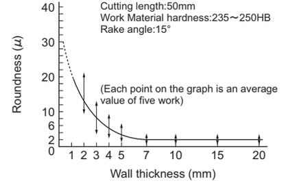
Fig.21-2 Relation between roundness and wall thickness
