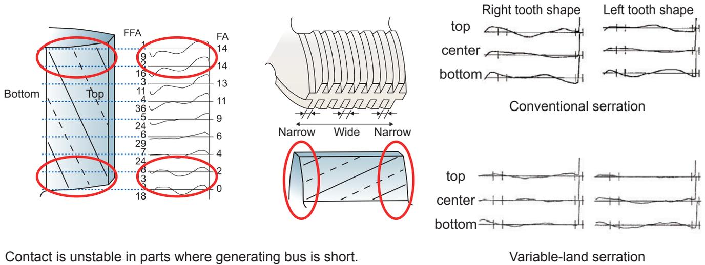
Contact is unstable in parts where generating bus is short.
