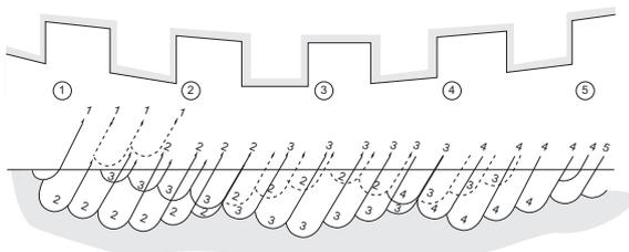
Nonuniform amount of cutting for each serration cutting blade
