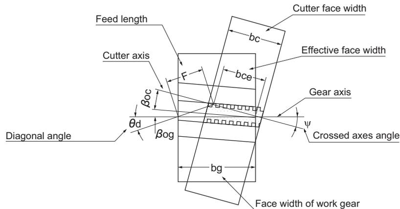
Fig.11 Relation of diagonal angle and face width
