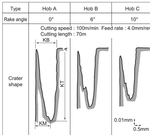
Fig.15 Craters of TiN coated hobs those which have different rake angle in spur gear cutting
