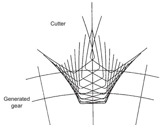
Fig.2 Generation of gear tooth profile by shaper cutter
