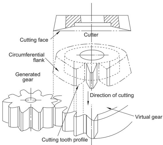
Fig.3 Gear cutting by spur type shaper cutter
