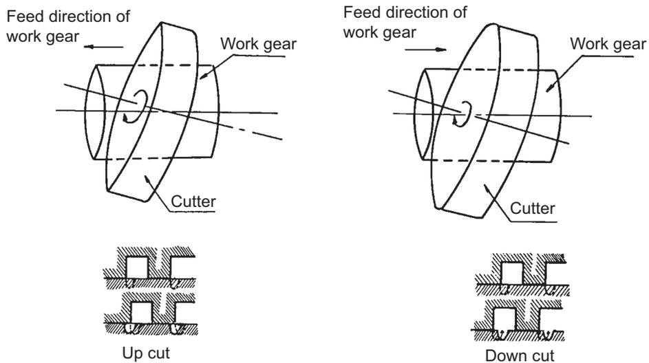
Fig.16 Action for cutting edge by rotational direction of cutter and traverse direction of work gear
