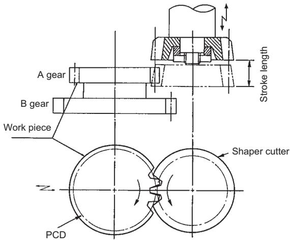
Fig.1 Gear cutting by shaper cutter
