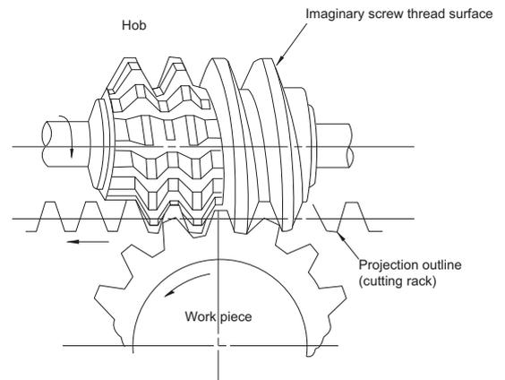
Fig.1 Gear cutting mechanism of hob
