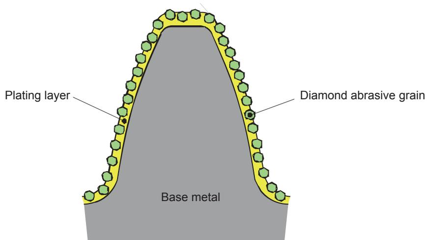
Fig. 2: Diamond dressing gear tooth construction
