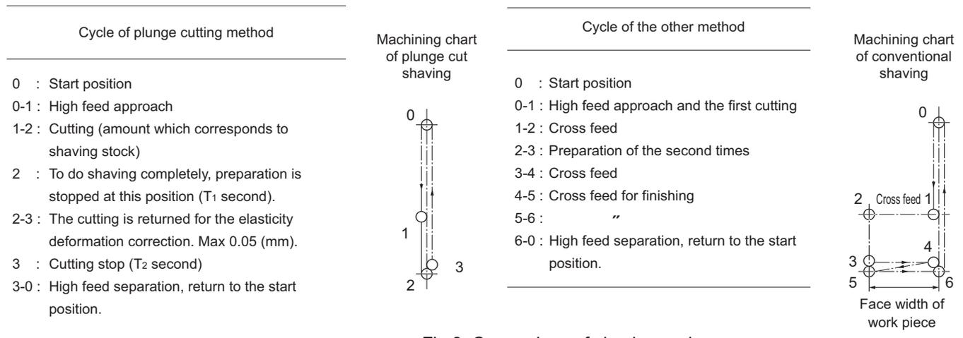
Fig.3 Comparison of shaving cycle
