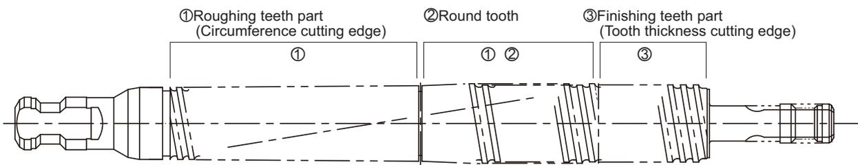
Fig.7 Integrated helical broach
