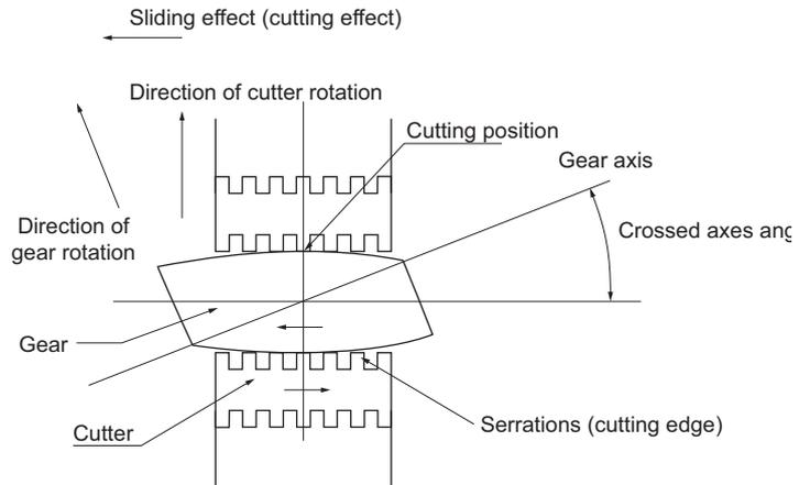
Fig.1-2 State of cutting action on the mating pitch cylinder
