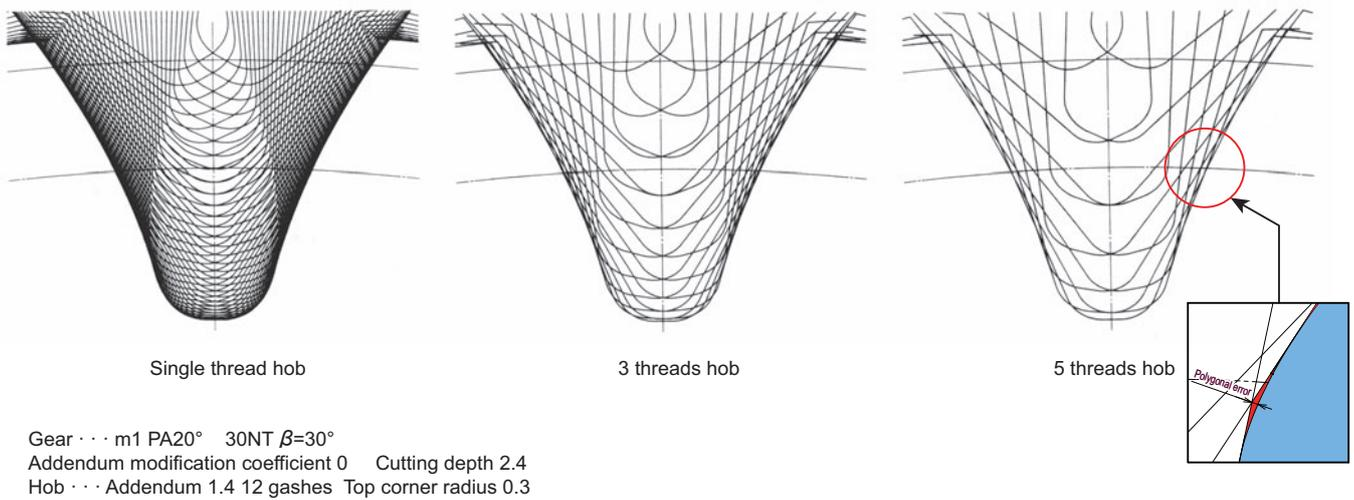
Fig.6 State of generation of multi-thread hob
