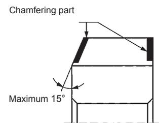
Fig.4 Gear whose end face inclines
