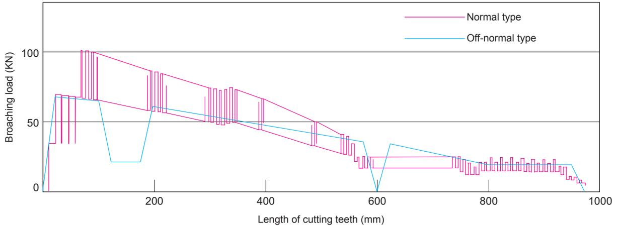
Fig.6 Comparison in broaching load
