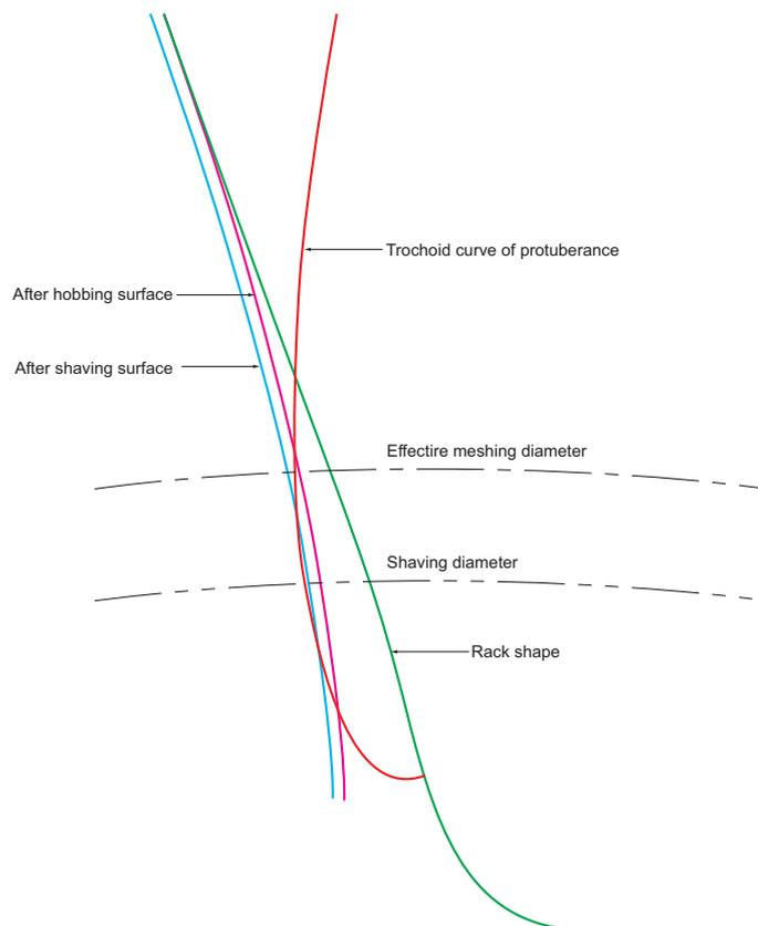
Fig.13 State of generation of tooth root of work piece
