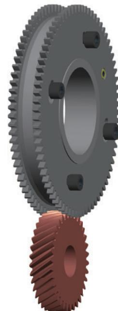
Fig. 2 Deburring cutter and gear
