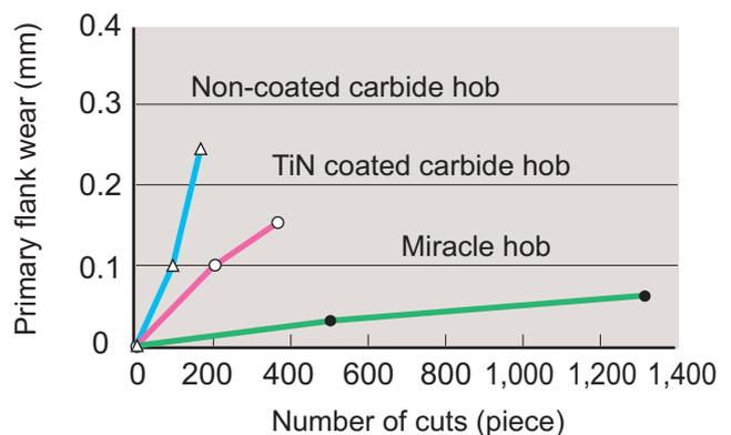
Fig.17 Comparison of the amount of wear in variety of coating
