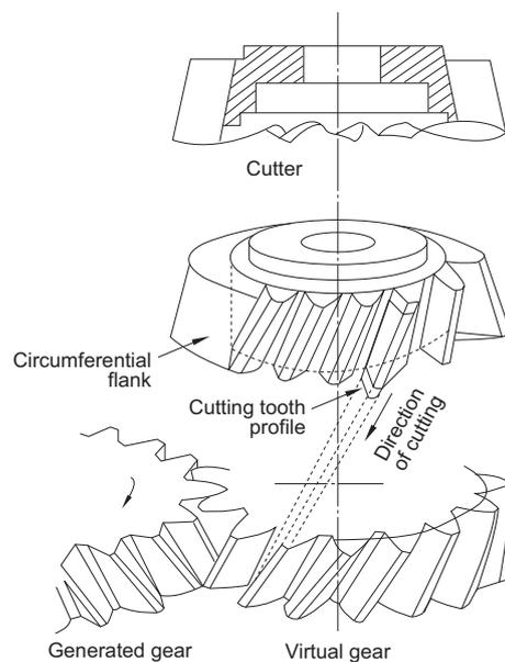
Fig.4 Gear cutting by helical type shaper cutter
