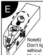
Screw: GY06013M Wrench: TKY30R Torque: 6.0 Nm
