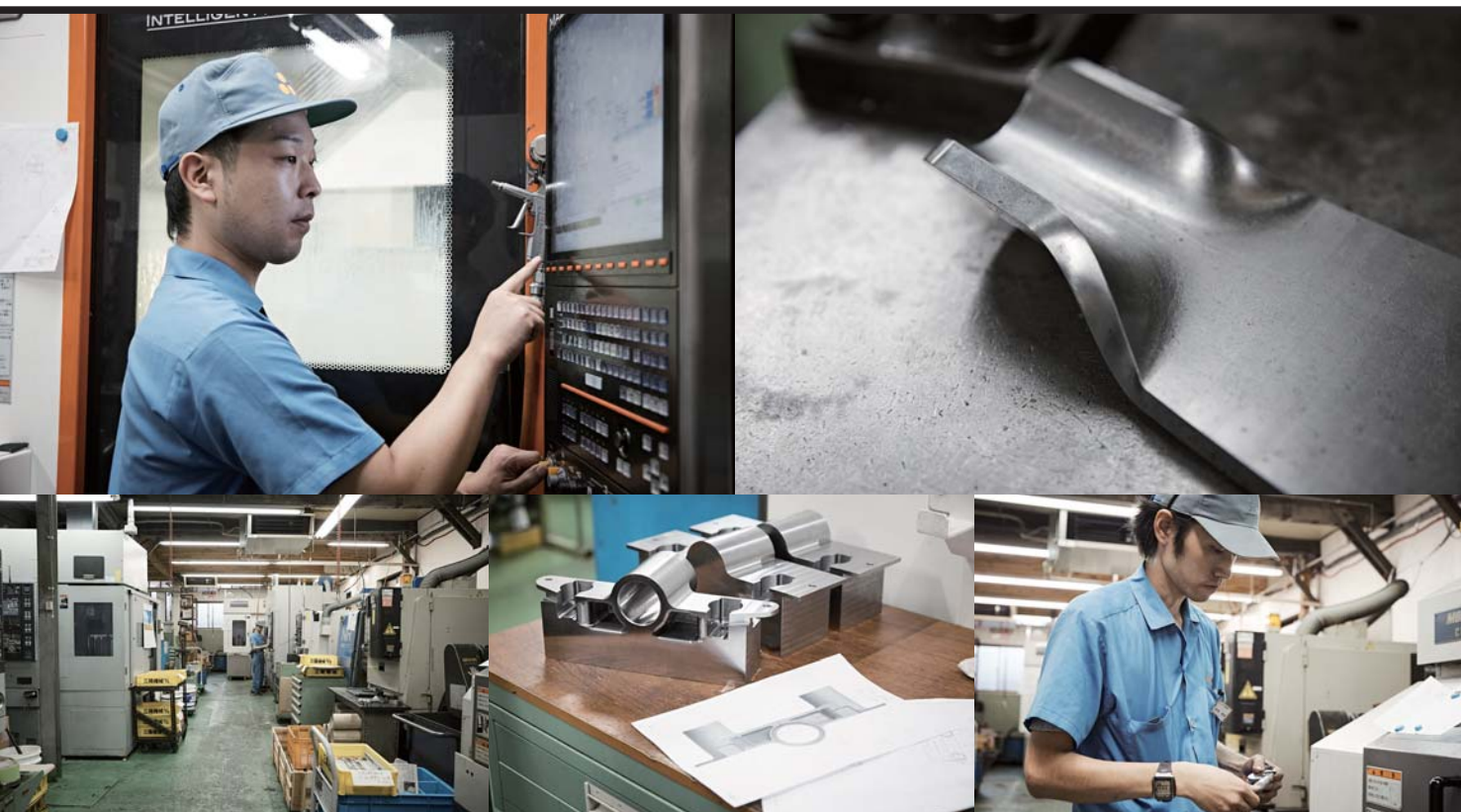
A small diameter radius end mill manufactured by Mitsubishi Materials was used for curved surface machining, and roughing type end mill was used for rough machining during the process of manufacturing Shitamachi bobsleighs.
