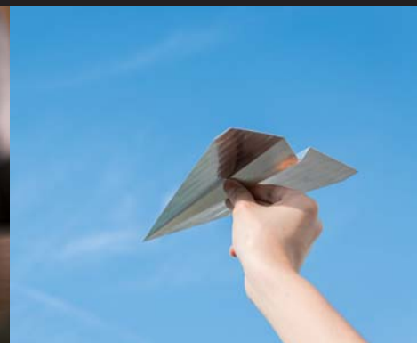
Only 0.2 mm thickness aluminium-made "paper" plane
