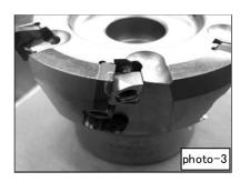
5. Loosen the screws of the cramping wedges and re-tighten them tightly.
