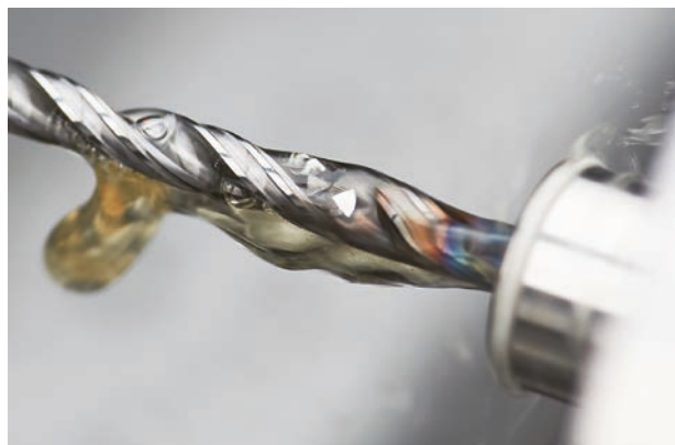
Chips generated by LFV
