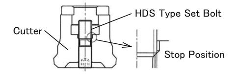
2Line up the key way of cutter, with that of the arbor without rotating the cutter tighten up the screw.
