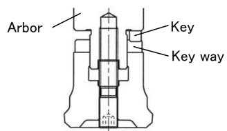
3 Ensure that the screw is tightly screwed into place, Then assembly is complete. Please ensure that the face connecting the spindle and the arbor is in full contact.
