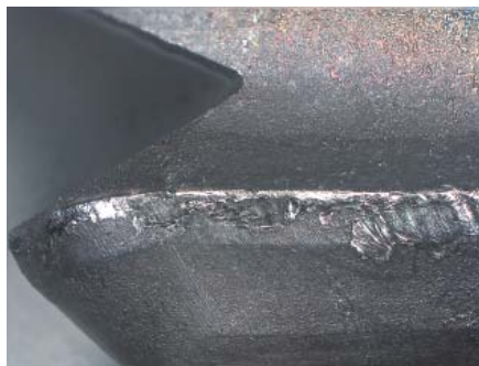
Condition of the edge after 30 m machining
