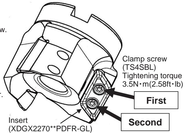
6. Ensure that there is no space between the insert and the insert seat.
