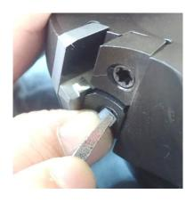
3 Push it into the hole further with flat head pin. Plug will stop at the upper part of wrench hole, since pin is wider than wrench hole.
