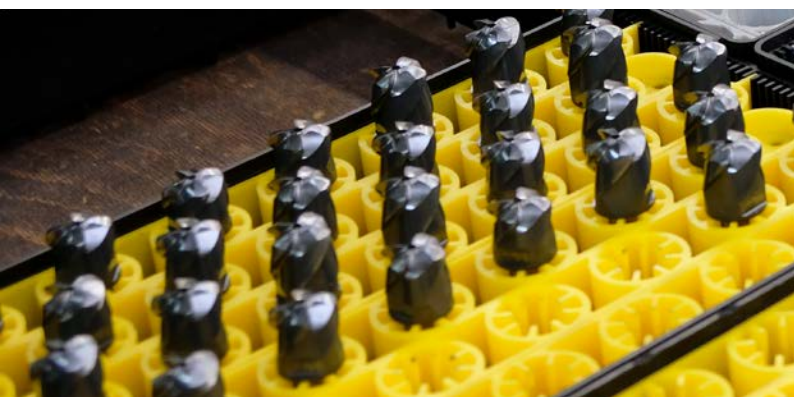
iMX tool heads in the re-grinding process
