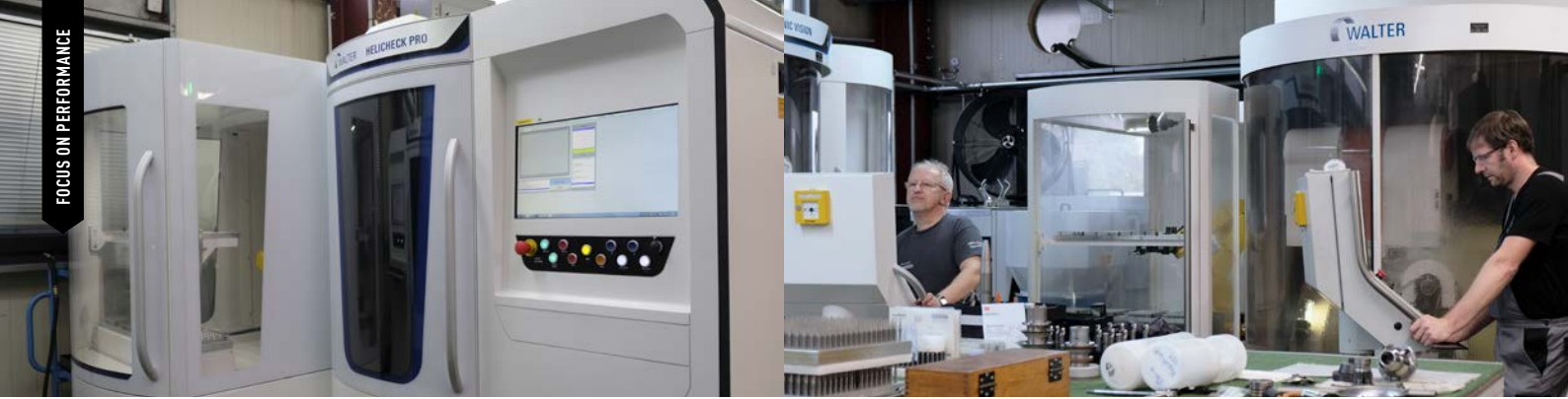
Helicheck Pro machine for fully automated measurement of tools
