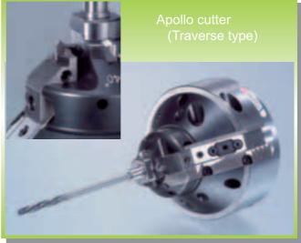
Cutting conditions vc=81.6m/min n=1,000min<sup>-1</sup> fr =0.05mm/rev vf=60mm/min ap=0.1mm/per side Wet
