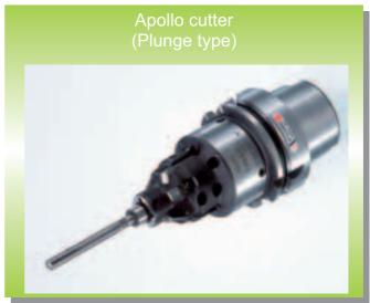
Cutting conditions vc=112.2m/min n=1,500min<sup>-1</sup> fr =0.12mm/rev vf=180mm/min ap=0.5mm/per side Wet
