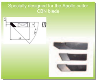
Cutting conditions vc=112.2m/min n=1,500min<sup>-1</sup> fr =0.12mm/rev vf=180mm/min ap=0.5mm Wet
