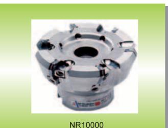
Cutting conditions vc=1,000-4,500m/min fz=0.05-0.30mm/tooth ap=0.3-3.5mm Wet
