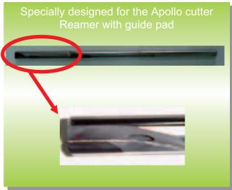
Cutting conditions vc=40m/min n=2,120min<sup>-1</sup> fr =0.12mm/rev Wet
