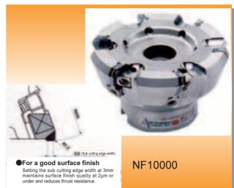
Cutting conditions vc=1,000-4,500m/min fz=0.05-0.20mm/tooth ap=0.3-2.0mm Dry
